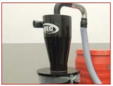
HEC Pre-Separator filters out submicron particles before they reach the vacuum's primary filter
